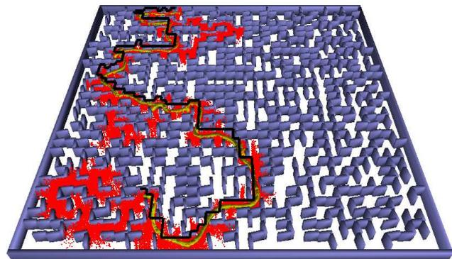
Fig. 1. Example of benchmark “RandomSlantedWalls,” a kinodynamic motion planning problem solved by DSLX two orders of magnitude faster than other tree-based motion planning methods. The robot model is that of a smooth car (see Section III-A). Red dots indicate projections of the states of the exploration tree onto the workspace. The black line indicates the current lead that is used to guide the tree exploration toward the goal.
