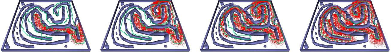
(b) Exploration of benchmark "WindingTunnels" after 2s, 4s, 6s, 8s of running time
