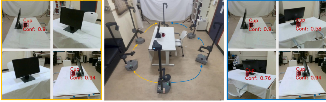
Figure 11. Real-robot cup-detection experiment: motion paths for Manifold-line (orange) and PS-PRM-line (blue), with camera views for each shown top-to-bottom, left-to-right.
