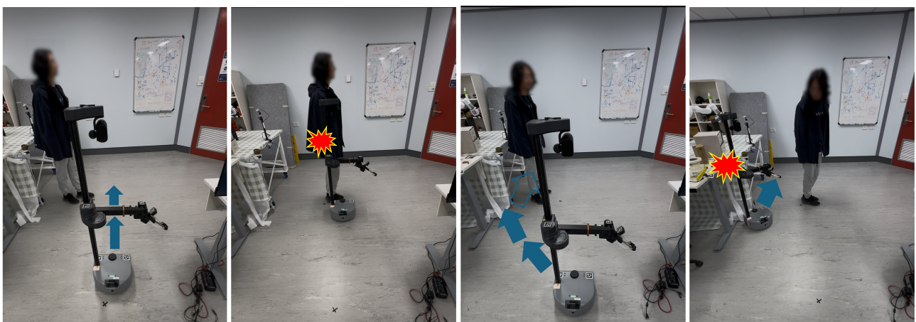
Figure 11. Stretch demonstrations for B-VAMP (first two pictures) and R-POMCP (last two pictures). B-VAMP moves forward and collide with the moving pedestrian due to lack of POMDP planning and R-POMCP tries to avoid the person but went too far and collided with the environment.
