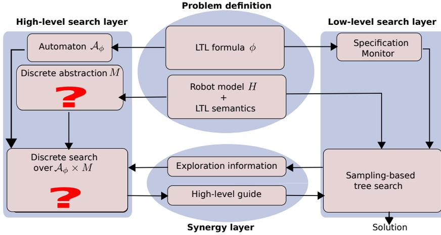
Fig. 3: Synergistic multi-layered approach for motion planning with LTL specifications
