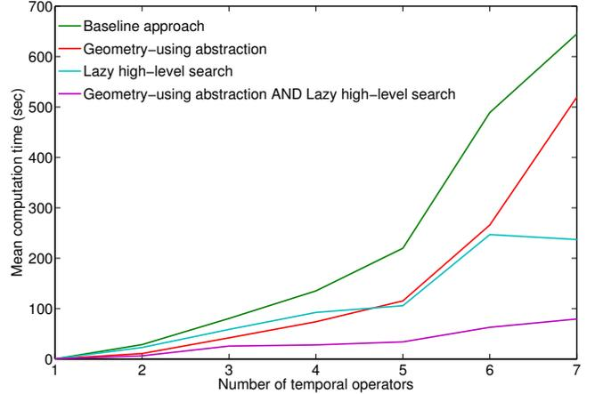
Fig. 7: A combination of geometry-using abstractions and lazy high-level search can result in speedups of close to 10 times when compared to the baseline approach. The baseline approach is the one that uses geometry-ignoring abstraction and reinitialized high-level search. See also Section II-D and [29].
