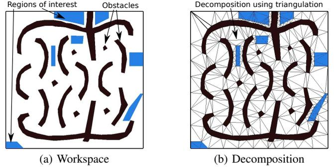
Fig. 5: (a) Workspace with seven propositions. The sets shown in blue are labeled with propositions. (b) Triangulation-based decomposition of the workspace. The triangulation-based decomposition was done using conforming Delaunay triangulation and resulted in 618 elements in the decomposition. See also Section II-B and [28].
